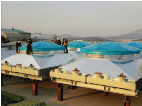
Air cooler (induced, forced type) preservation for long term outdoor storage and transportation with VpCI-126® High Performance UV Film .
